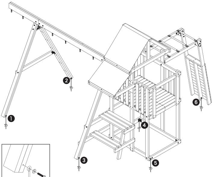
Note: If soil conditions permit anchors to be pulled out easily, such as in sandy soil conditions, cementing is required. If your ground is too hard to screw in the anchors you can remove the earth with a shovel. Install the anchors and compact the earth as you replace it. Anchors must be placed below the level of the shock-absorbing surfacing material to prevent tripping or injury resulting from a fall.
