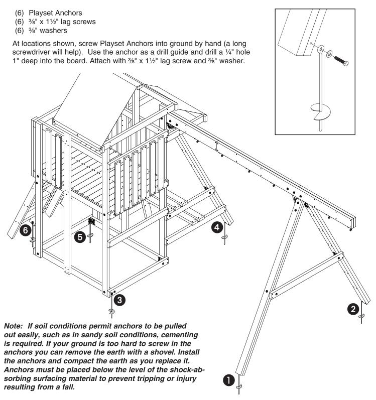
Reminder: Be sure to install proper shock-absorbing surfacing material. Refer to the Safety Guidelines at the beginning of this plan.
