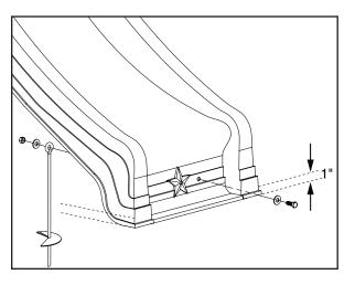
Caution: Failure to anchor the Slide properly could cause serious injury from children lifting the Slide.
